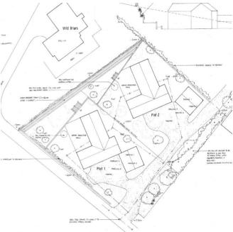
3.2 The dwellings would be c. 14 m wide for 6.3 m back with a 10.5 m projection at the rear that is c. 6.3 m wide. In terms of height, they would be 5.3 m to the eaves and 8 m to the ridge. The double garages each measure c. 6.7 m x 7.2 m, 2.5 m to the eaves and 5.3 m to the ridge.
